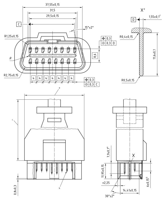
Figure A.2 — Type A external test equipment connector
