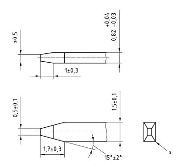
Dimensions of the  $1,5 \times 0,8$  blade according to ISO 8092-3 are also acceptable.
