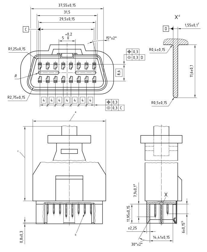
Figure B.2 — External test equipment connector Type B
